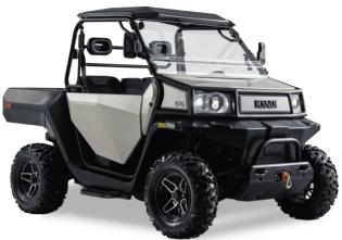
The Wombat UTV is a powerful electric vehicle with an AWD system that enables off-road driving for different terrains. This vehicle comes fully equipped with a winch that can pull 1500 kg and an electric dump tray that has a 500 kg maximum capacity. This vehicle is ideal for farms, acreages, parks, and private properties.
