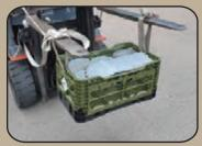
Weight Capacity 440lbs(200kg) Static Capacity 2200lbs(1000kg)
