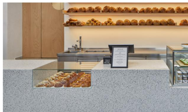
Staron Solid Surfaces is manufactured from a safe natural mineral refined from bauxite and blended with pure acrylic resin. A non-porous material, Staron provides a hygienic, durable and easy to maintain surface.
