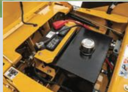
Heavy-Duty Hydraulics With 11 litre oil reservoir, oil cooler w/ fan & hot oil shuttle.
